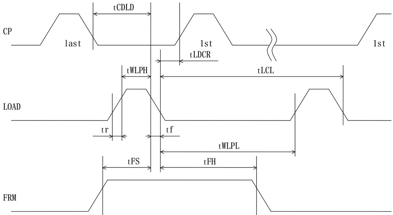
10-1. Switching characteristics ( $V_{DD} = 5.0V$ )
